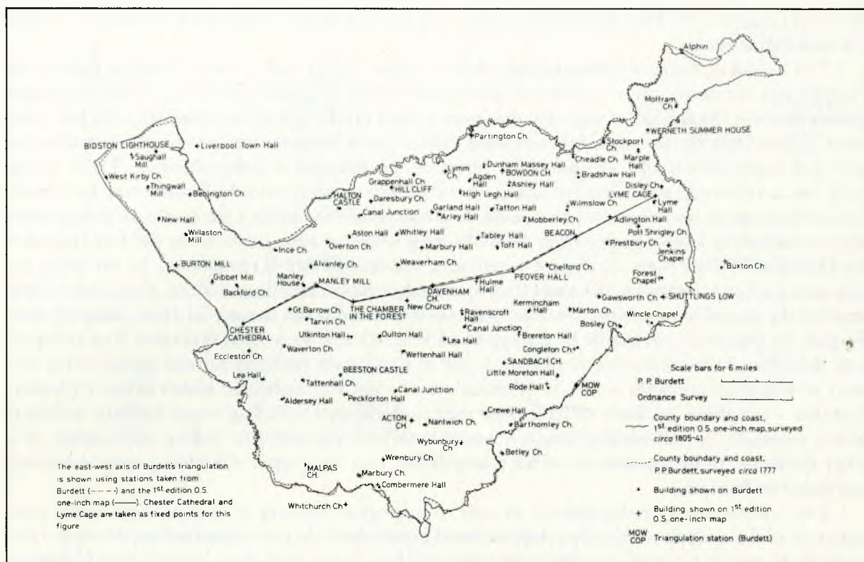
Figure 3. Burdett's geodetic survey. 101 randomly selected features in addition to the triangulation stations in the county are shown in relation to their positions on the first series of the Ordnance Survey. The excellent coincidence of the county boundary with only a few major deviations should be noted.
